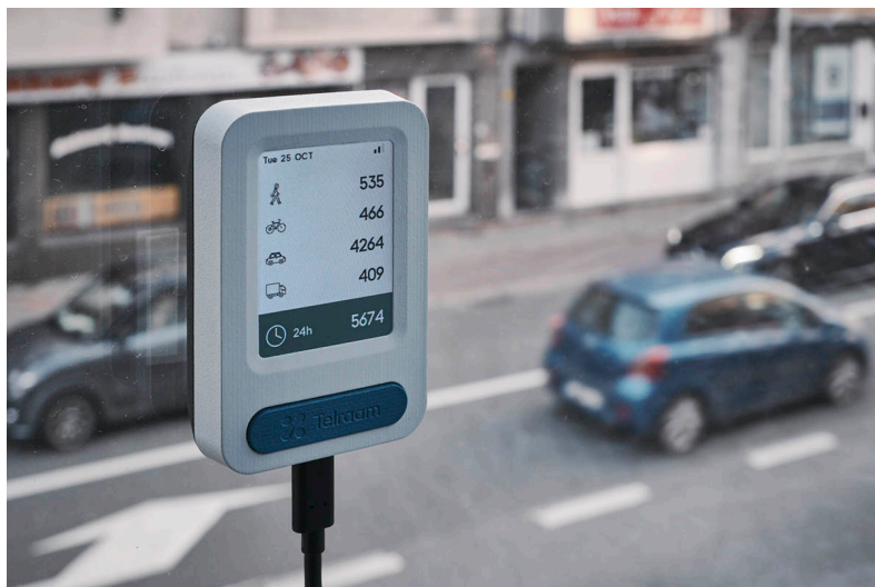
Figure 11 Indoor and outdoor smart traffic count devices
