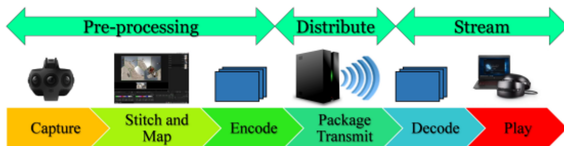
Figure 5 End-to-End 360-degree video streaming framework.
