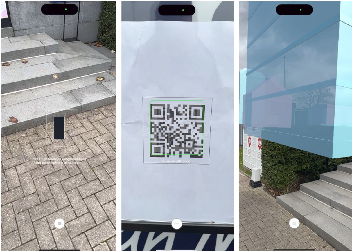
Figure 2: To test the Tool A procedure, a QR code was installed at the entrance of the pilot site (see middle image), allowing users to launch the tool on a smartphone or tablet. Subsequently, users are instructed to move their device for calibration purposes (see left image), ensuring that the buildings are correctly positioned within the AR environment for a full immersive experience (see right image).
